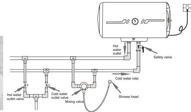
(Figure 3) for reference in installation only
