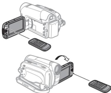
**Point the controller at the camcorder's remote sensor when you press the buttons.**
