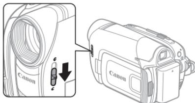
Move the lens cover switch down to to open the lens cover.
