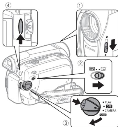
**1** Move the lens cover switch down to ☞ to open the lens cover.
