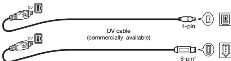
\* Be careful to correctly insert the 6-pin plug into the DV terminal. Inserting it in the wrong direction can result in damage to the camcorder.
