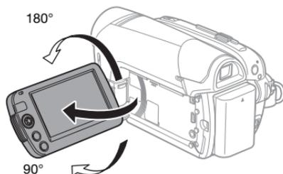
You can rotate the panel 180 degrees toward the lens (allowing the subject to monitor the LCD screen while you use the viewfinder). This is the only case where you can use the viewfinder and
