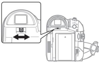
Adjust the viewfinder as necessary with the dioptic adjustment lever.
