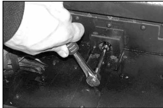
Figure 14: Removing the orifice.
