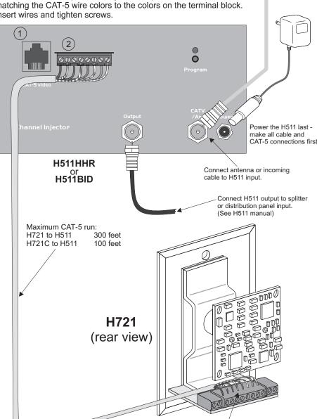
Insert wire into terminal block and tighten screws. Use the color bar to match wire colors. The color bar has two rows, one for CAT-5 and one for quad wire:
