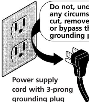
Power supply cord with 3-prong grounding plug
