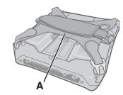
When using the computer holding with hand, insert your hand to (A) part of the hand strap. Fix the hand strap firmly so that the computer does not come off, and then turn it over.
