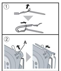
We recommend you fix the stylus in safe to the computer using the tether (supplied).
