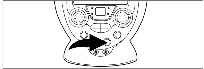
When the vocal feature is activated, the vocals on a multiplex recording are muted as soon as the singer begins singing into the microphone. When the singer stops singing, the vocals are automatically unmuted. Adjust the AVC control for the best balance between playback and microphone levels.
