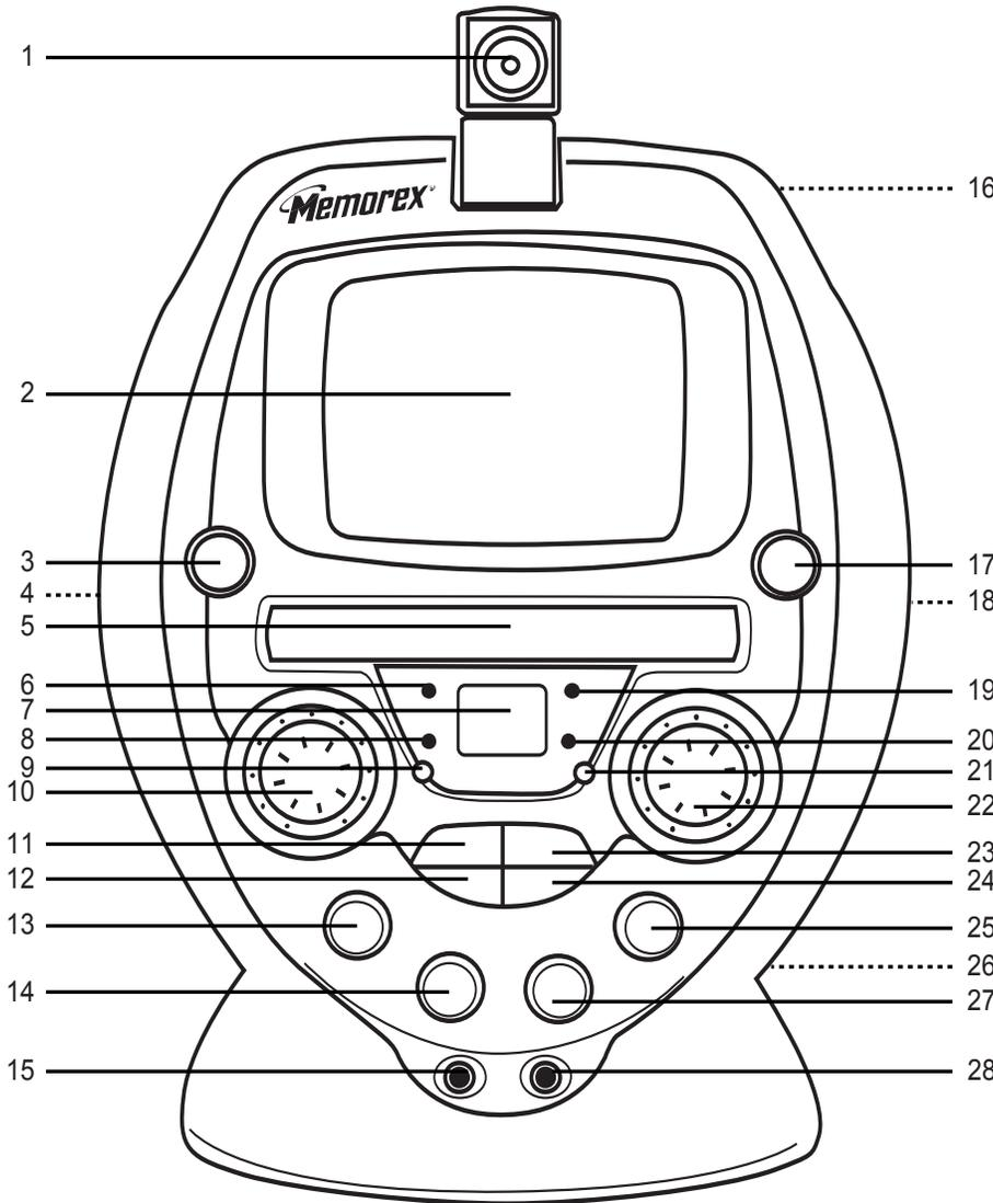
1. Video Camera with Camera Focus Adjusting Ring
