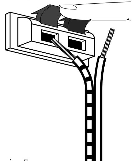
4. Twist the tiny strands in each conductor into tight spirals, as shown in Drawing 4.
