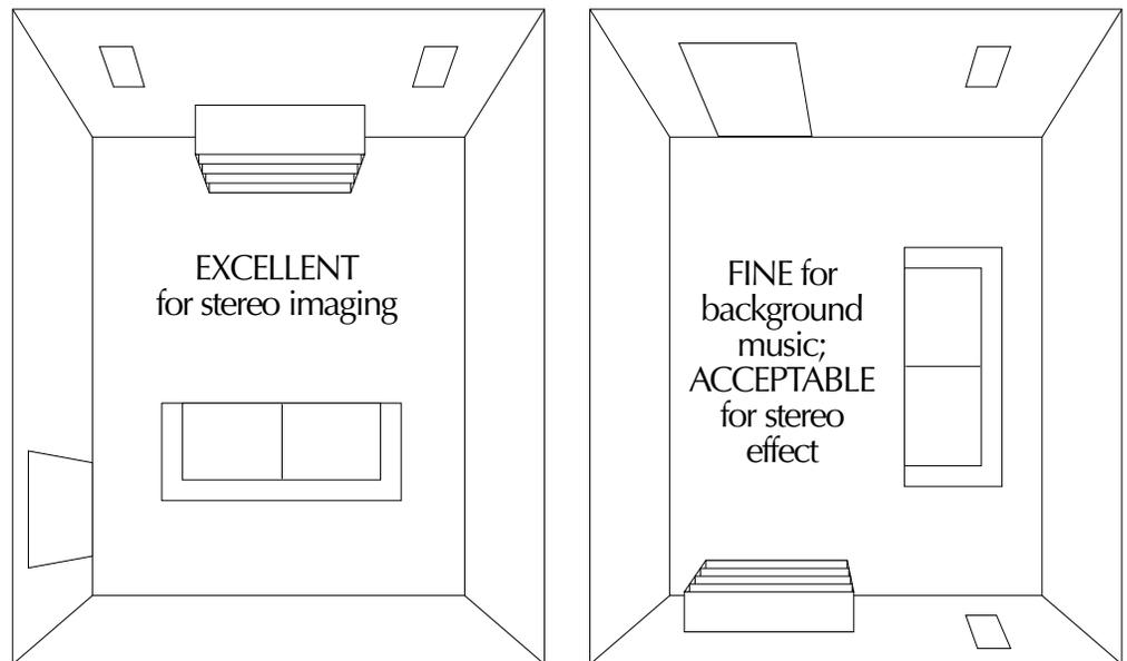
Russound In-wall speakers may be used for rear surround sound channels by placing them (1) behind, (2) on each side of the viewing position or (3) in the ceiling just behind the viewers. The SP550.2 & SP650.1 speakers also make excellent, unobtrusive front channel home theater speakers for 5 channel listening.
