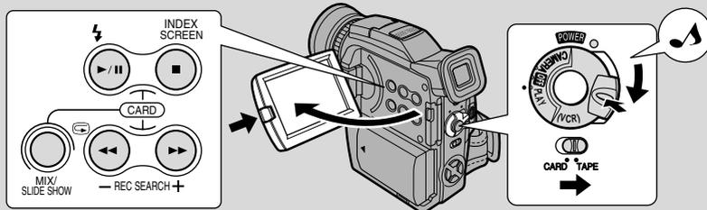
You can use the LCD screen for instant, on-the-spot playback. The camcorder also plays back the sound track via the built-in speaker ( 35).
