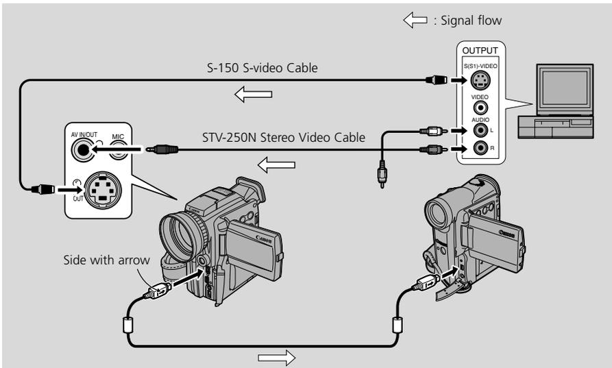
Above illustration shows the connection using a S-video cable. You can also connect to the VIDEO terminal instead ( 38).
