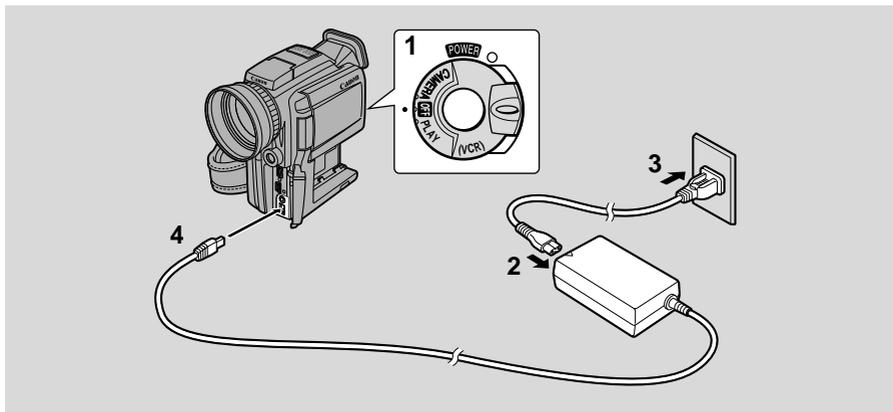
Use the power adapter to provide your camcorder with instant power from a household power socket. Always turn the camcorder off before connecting/removing the power source.
