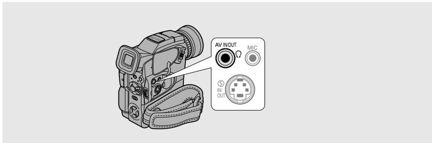
Through the menu, the camcorder's AV/headphone terminal can be switched to function as either the AV terminal or the headphone terminal.
