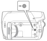
Connect the external microphone to the MIC terminal. Use commercially available condenser microphones with their own power supply and a cable no longer than 3 m. You can connect almost any stereo microphone with a Ø 3.5 mm plug but audio recording levels may vary.
