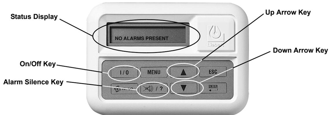
Active alarms are displayed on the LCD screen and sound an audible beep. To silence an alarm, press the Alarm Silence/Help key as prompted on the display.
