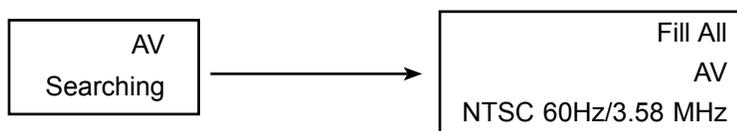
When there is no signal from the selected source (see illustration), either change the channel or press **Source** button to change sources. If there is no signal on your selected source for 15 minutes the television will power down.
