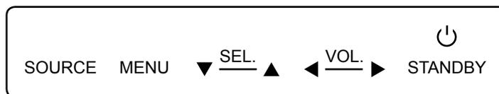
**SOURCE:** Press to display the source menu, Use ▲ or ▼ button to select AV, S-Video, YPbPr 1, YPbPr 2, VGA or HDMI, then press ► button to confirm.
