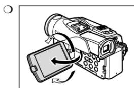
You can rotate the LCD panel. Make sure to open the LCD panel at 90 degrees before rotating it.
