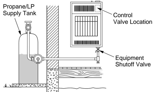
Figure 16 - Checking Gas Joints for Propane/LP Gas
