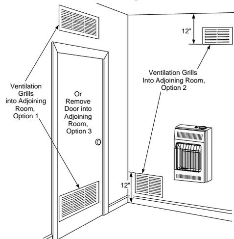
Figure 2 - Ventilation Air from Inside Building
