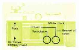
around the spool, take the slack out of the film and check to see that film perforations are accurately engaged on the spool sprockets.
