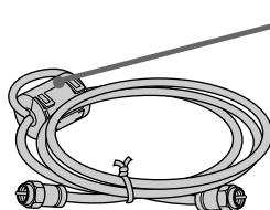
Do not detach the ferrite core from the cable.
