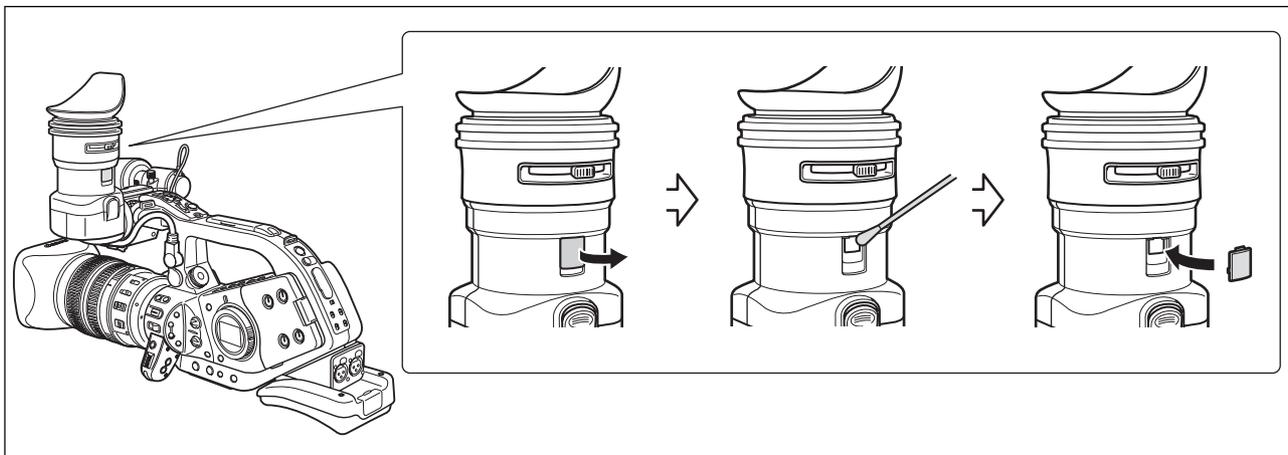
1. Open the protect cover (e.g. using a flathead screwdriver).
