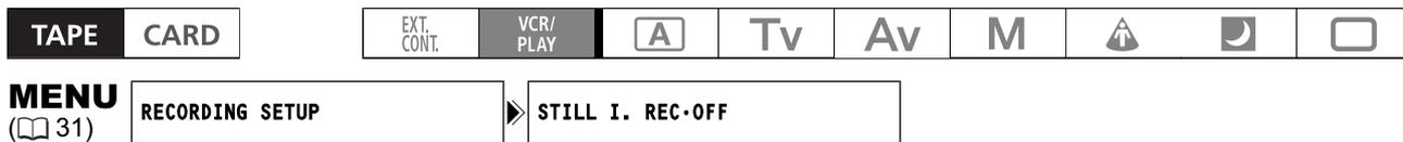
1. Open the menu and select [RECORDING SETUP]. Select [STILL I.REC], set it to [ON] or [ON+CP DATA] and close the menu.
