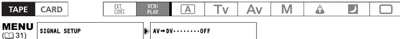
Open the menu and select [SIGNAL SETUP]. Select [AV→DV], set it to [ON] and close the menu.
