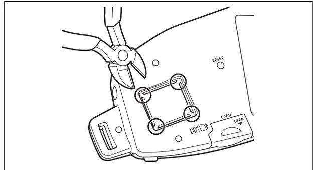
3. Using a pair of pliers extract the flexible board on which the lithium battery is installed and pull to detach it.
