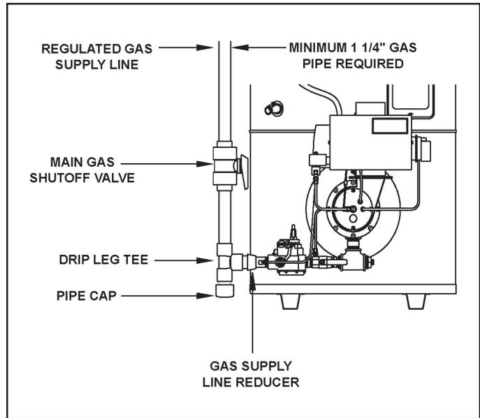
**GAS PIPING AND DIRT LEG INSTALLATION**
