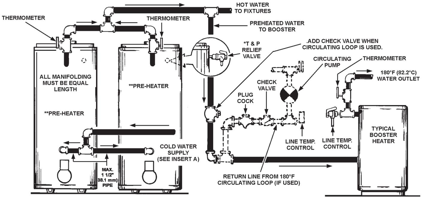
CAUTION: IF BUILDING COLD WATER SUPPLY HAS A BACKFLOW PREVENTER, CHECK VALVE OR WATER METER WITH CHECK VALVE, PROVISIONS FOR THERMAL EXPANSION OF WATER IN THE HOT WATER SYSTEM MUST BE PROVIDED.
