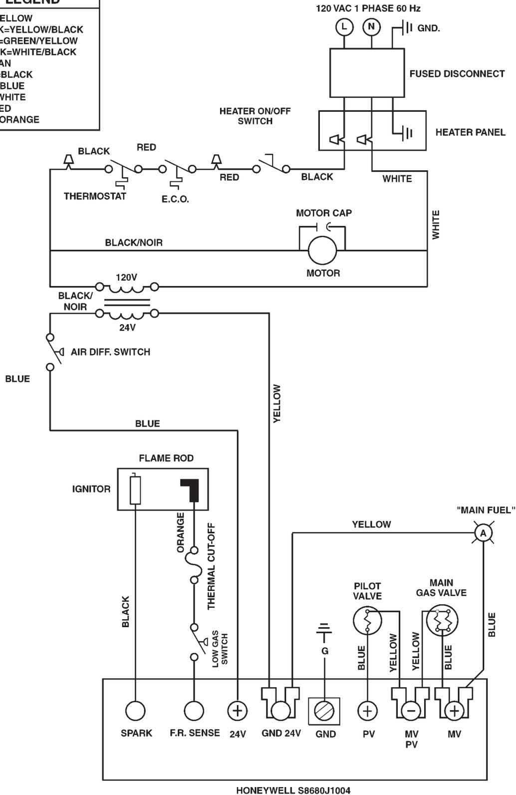
**WIRING DIAGRAM FOR COMMERCIAL LOWNOX WATER HEATER FROM BAROMETRIC VENT**
