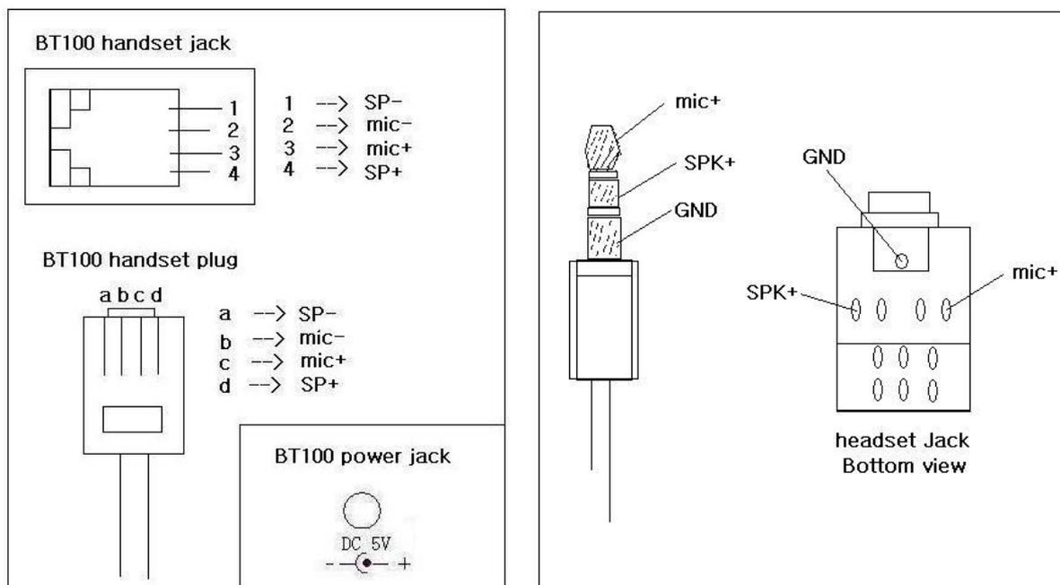
**NOTE:** For GXP-2000 HW REV. 0.3 and 0.4, a 3.5mm to 2.5mm plug converter is required to use a 2.5mm headset. The converter can be purchased at any electronics store.
