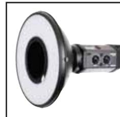
This is an accessory to the 75° Softlite reflector that creates a unique lighting effect by including a Perspex outer diffuser with a honeycomb and grid in the centre. The Grid Diffuser gives a pool of direct light in the centre of the image, surrounded by soft-diffused light. The ratio between the centre and edge is 3:1 - ideal for portrait applications. **BW1866**
