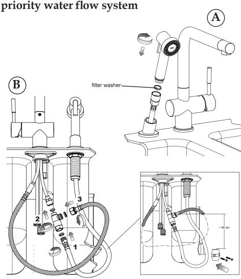
Proceed to the connection of the flexible hose of the side spray (A) and the priority water flow system (B - follow the phases indicated). Interposing the holding gaskets within the connections as indicated in the figure. Fix the lead counter weight to the flexible hose of the side spray at a distance of approx. 40 cm from the connection to the outlet pipe.
