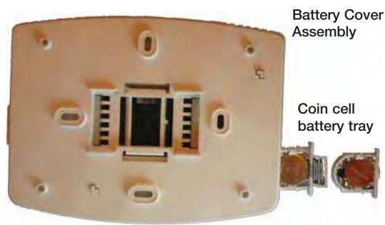
Insert the coin cell battery in the coin cell battery tray and push it inside the battery cover assembly
