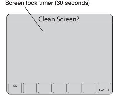
Press **SCREEN** to go to the cleaning screen. Press **OK** to lock the screen for cleaning. The screen remains locked for 30 seconds so you can clean the screen without disturbing any settings.
