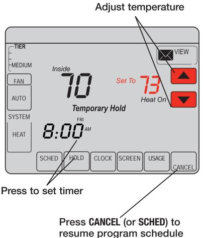
Press ▲ or ▼ to immediately adjust the temperature. This temporarily overrides the temperature setting for the current time period.
