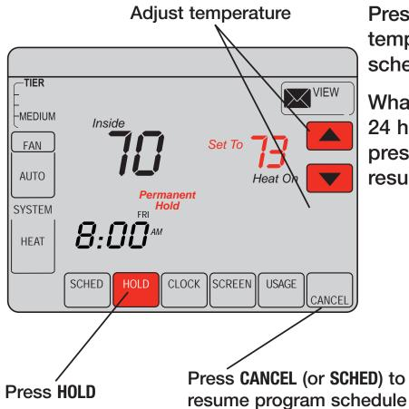
Press **HOLD** to permanently adjust the temperature. This turns off the program schedule.
