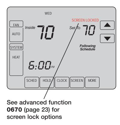
To prevent tampering, the screen can be partially or fully locked.
