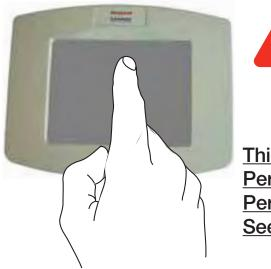
BE CAREFUL! Never use sharp instruments, such as a pencil or pen, to press touchscreen keys. To prevent damage to the thermostat, always press keys with your fingertip.
