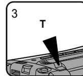
3. When you move the ZOOM lever to "T" side, the picture will increase in size upto a maximum of 880 times. (VP-W75D: 990x)
