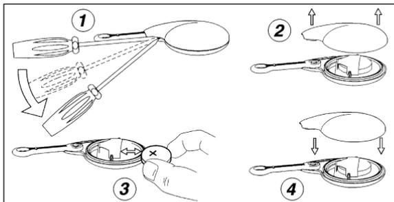
3. Wait for 10 seconds before inserting the new battery, ensuring the correct polarity (+ sign upwards) and holding the battery by the edge.
