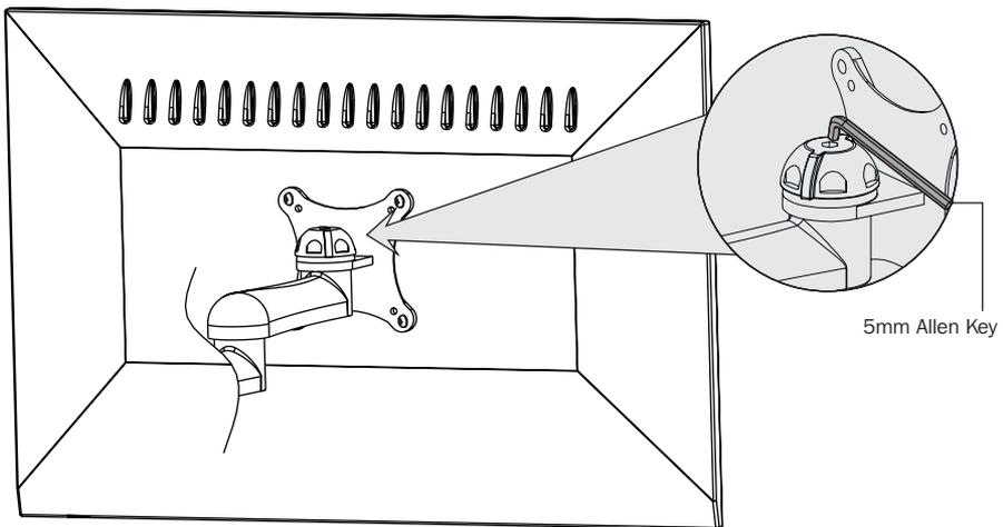
Tighten the adjustment screw by using Allen Key provided to fix the tilting angle
