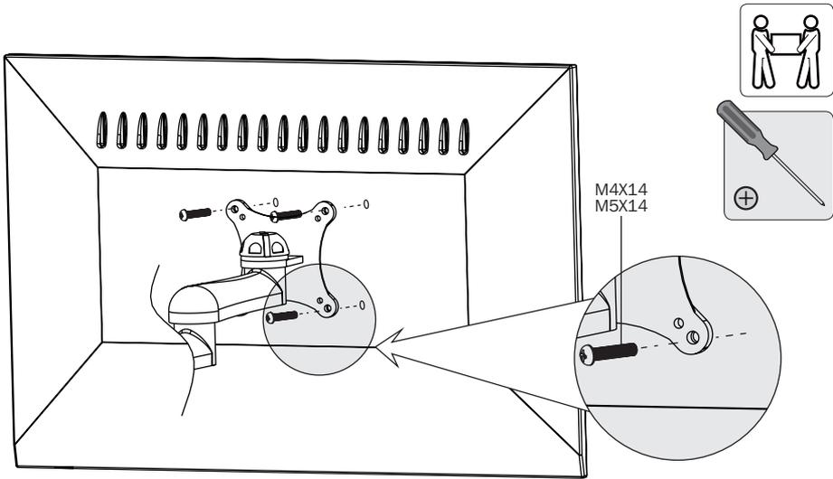
Lift the display and match the holes on your display with the holes on the mount. Secure your display to the mount by tightening screws
