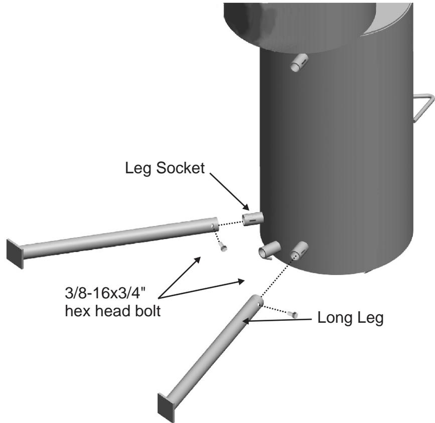
**4** Attach short legs to remaining leg sockets near firebox using **3/8-16x3/4" hex-head bolts**. Do not fully tighten. Tighten bolt just enough to keep leg from sliding off of socket .
