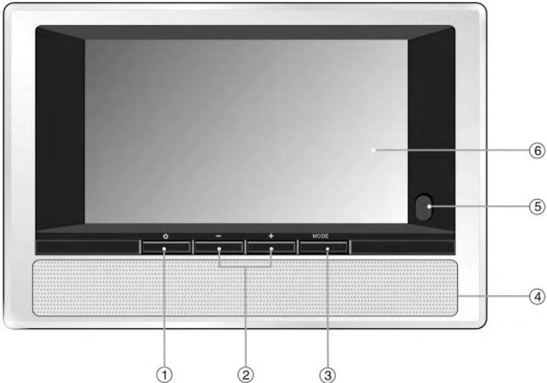
1. **POWER button:** press to access or to exit the standby mode
