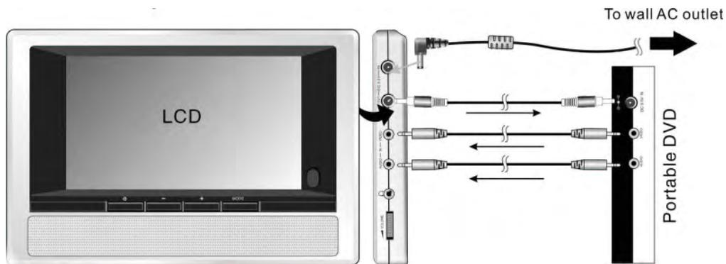
Note: the AC adapter must connect to the extra screen or it will not have power.
