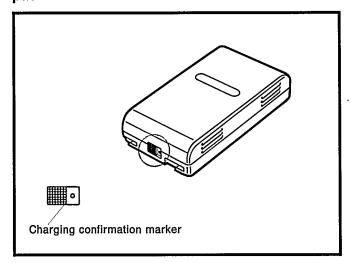
This marker makes it convenient to distinguish between charged and discharged battery packs. For example, visible dot means charged battery pack, and no dot means discharged battery pack.
