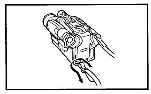
Attach the other end of the shoulder strap at the lower part of the rear of the Camcorder in the same way as mentioned above.
