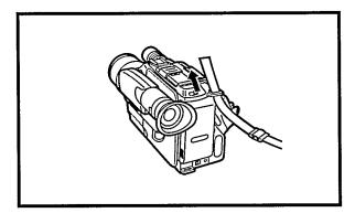
Pass the end of the shoulder strap through the slit of the shoulder strap holder on the upper part of the rear of the Camcorder.
