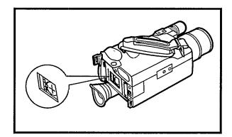
Insert the "CR2032" size battery with polarities (+ and -) aligned correctly and then replace the lid.
