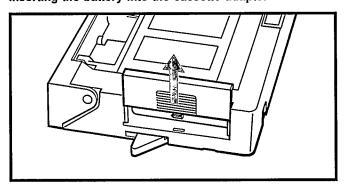
Remove the battery cover by sliding it up. Install one "R6" battery and reattach the cover.
