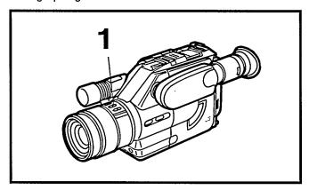
**1** By repeatedly pushing the SHUTTER button, the shutter speed can be changed as follows:
