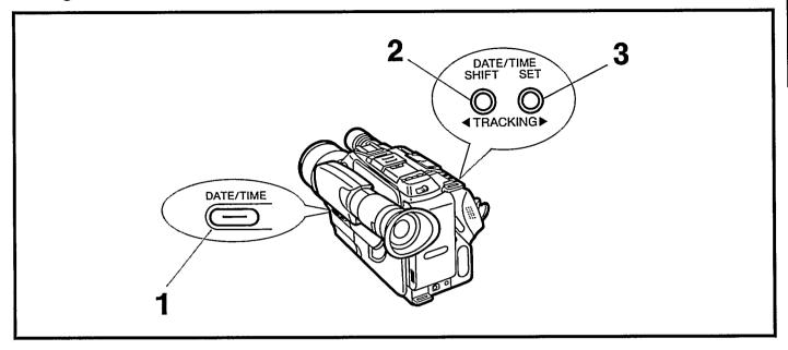
1 When the DATE/TIME selector button is pushed, the indication shown below will appear in the EVF.
