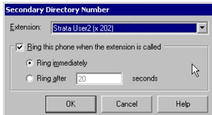
The Secondary Directory Number dialog box has a title bar "Secondary Directory Number". It contains an "Extension:" dropdown menu with "Strata User2 (x 202)" selected. Below it is a checked checkbox "Ring this phone when the extension is called". Under this checkbox are two radio buttons: "Ring immediately" (selected) and "Ring after" (with a text field containing "20" and the word "seconds" to its right). At the bottom are "OK", "Cancel", and "Help" buttons.
