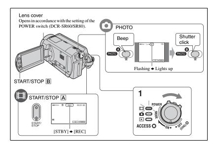
1 Slide the POWER switch in the direction of the arrow repeatedly until the respective lamp lights up.
