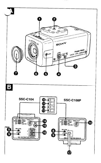
screw hole to fix the camera to a mounting bracket. The mounting screw must be of the following type.
