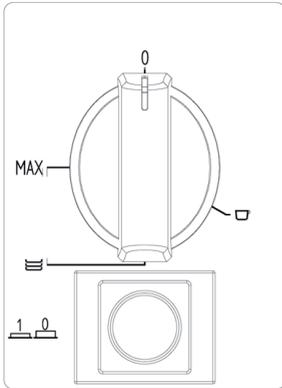
The control elements are the temperature knob and the luminous ON-OFF switch.
