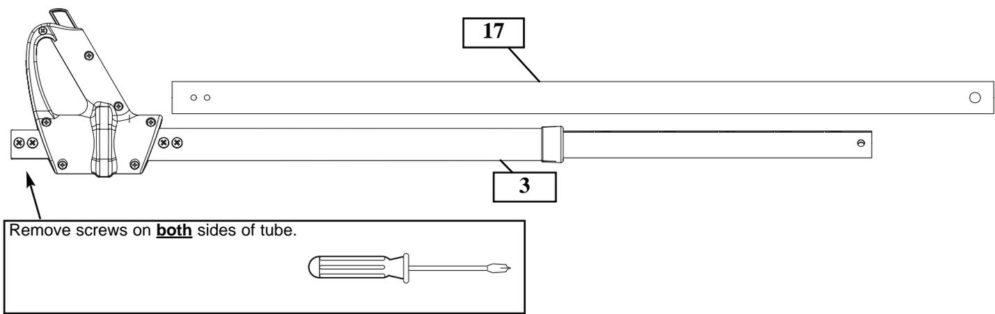
**6.** Slide upper tube (17) onto handle assembly (3). Reinsert screws removed in previous step as shown.
