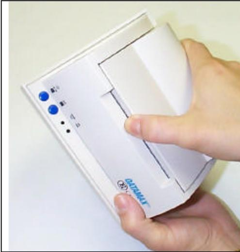
Option #3. Hold the base of the E-3202 in one hand. Using the other hand, place your fingers against the back of the paper bay door. Using your thumb on the front edge of the paper bay door, pull the door open.
