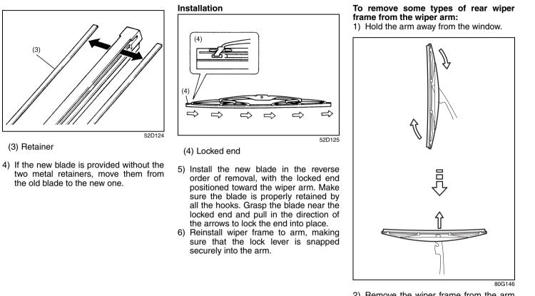
2) Remove the wiper frame from the arm as shown.
