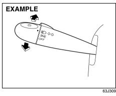
With the headlights on, push the lever forward to switch to the high beams (main beams) or pull the lever toward you to switch to the low beams. When the high beams (main beams) are on, a light on the instrument panel will come on. To momentarily activate the high beams (main beams) as a passing signal, pull the lever slightly toward you and release it when you have completed the signal.
