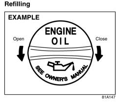
Remove the oil filler cap and pour oil slowly through the filler hole to bring the oil level to the upper limit on the dipstick. Be careful not to overfill. Too much oil is almost as bad as too little oil. After refilling, start the engine and allow it to idle for about a minute. Stop the engine, wait about 5 minutes and check the oil level again.
