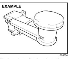
Check the brake fluid level by looking at the reservoir in the engine compartment. Check that the fluid level is between the "MAX" and "MIN" lines. If the brake fluid level is near the "MIN" line, fill it up to the "MAX" line with SAE J1703 or DOT3 brake fluid.
