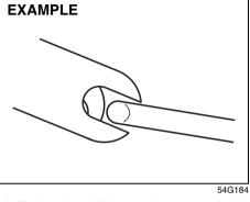
4) Push the child restraint toward the anchors so that the connecting bar tips are partially hooked to the anchors. Use your hands to confirm the position.
