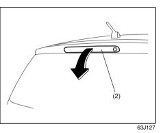
2) Close the tailgate. Remove a highmounted stop light housing (2) from the tailgate.
