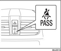
When the driver and front passenger don't buckle their seat belts, the driver's seat belt reminder light in the instrument cluster and the front passenger's seat belt reminder light in the information display will come on and a buzzer will sound as a reminder to the driver and front passenger to buckle their seat belts.
