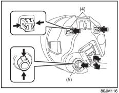
4) Open the fender cover. Disconnect the coupler by pushing the lock release. Pinch both side of the clips (4) and (5), and push them in.
