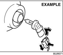
Open the fender cover. Disconnect the coupler with pushing the lock release. Turn the bulb holder counterclockwise and remove it. Rear combination light (tail, stop, turn signal, etc.)
