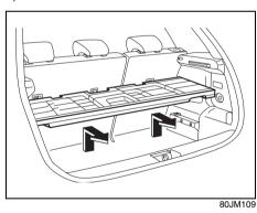
2) Lift the board, and remove the board from the vehicle.
