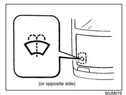
Check that there is washer fluid in the tank by looking at the washer fluid level gauge which is attached to the cap of the washer fluid tank. If the fluid level is near "E" mark, refill it.
