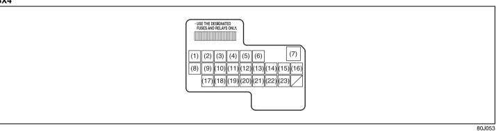
FUSE NAME PROTECTED CIRCUIT COLOR/SIZE (AMPS) **RR WIP** (1) **BLUE (15)** Rear wiper IG COIL (2) BLUE (15) Ignition coil RED (10) Back-up light (3) BACK MTR (4) RED (10) Meter ACC (5) **BLUE (15)** Accessory Under the FUSE dashboard ACC2 (6) BLUE (15) Accessory 2 BOX P/W (7) PINK (30) Power window WIP (8) **GREEN (30)** Wiper IG1 SIG IG1 SIG (9) RED (10) (10) **BLUE (15)** A/B Air bag RED (10) ABS (11)Anti-lock brake system
