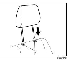
To reinstall the head restraint, insert the
