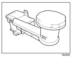
Check the clutch pedal for smooth operation and clutch fluid level from time to time. If clutch dragging is felt with the pedal fully depressed, have the clutch inspected by your SUZUKI dealer. If the clutch fluid level is near the "MIN" line, fill it up to the "MAX" line with SAE J1703 or DOT3 brake fluid.
