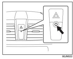
This light will blink with the ignition switch in the "OFF" or "ACC" position. The blinking light is intended to deter theft by leading others to believe that the vehicle is equipped with a security system.
