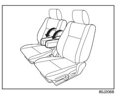
To use the armrest, pivot it down from the stowed (fully up) position. When not in use, return the armrest to the stowed position.
