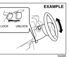
The lock lever is located under the steering column. To adjust the steering wheel height:
