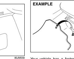
Your vehicle has a fastener to keep the driver's side floor mat from sliding forward and possibly interfering with the pedals. Whenever you put the driver's side floor mat back in the vehicle after it has been removed, be sure to hook the floor mat grommet(s) to the fastener(s) and position the floor mat properly in the footwell.
