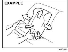
Make sure the child restraint is securely fastened by trying to move the child restraint system in all directions, especially forward.
