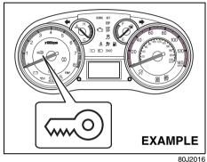
If the remote controller is not in the vehicle under the following conditions, a buzzer sounds intermittently for about 2 seconds and the keyless start system indicator light on the instrument cluster blinks in red:
