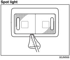
Pull down the lens by using a flat blade screwdriver covered with a soft cloth as shown. To install it, simply push it back in.
