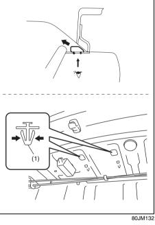
To remove the high-mounted stop light housing, pinch both side of the clip (1) and push it in.
