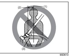
(1) Center of body(2) Less than 152 mm (6 inches)(3) Open end of extender buckle
