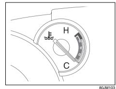
When the ignition switch is in the "ON" position, this gauge indicates the engine coolant temperature. Under normal driving conditions, the indicator should stay within the normal, acceptable temperature range between "H" and "C". If the indicator approaches "H", overheating is indicated. Follow the instructions for engine overheating in the "EMERGENCY SERVICE" section.
