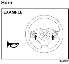
Press the horn pad on the steering wheel to sound the horn. The horn will sound with the ignition switch in any position.
