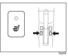
With the ignition switch in the "ON" position, push in one or both of the seat heater switches to warm the corresponding seat(s). The indicator light below the switch will also come on. To turn off the seat heater, push in the switch again. The indicator light below the switch will go off.
