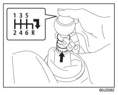
Reverse gear: with lifting up ring, shift the gearshift lever to the right, engage gear.
