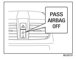
When the ignition switch is turned to the "ON" position, the "PASS AIR BAG OFF" indicator comes on for several seconds to let you know the system is working. When the front passenger sensing system has turned off the front passenger's front air bag including the seat belt pretensioner, the "PASS AIR BAG OFF" indicator will come on and stay on to remind you that the front passenger's front air bag is off.
