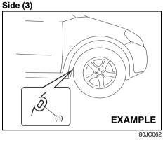
Frame hooks are provided on the front (1), rear (2) and side (3) of the vehicle. The hooks (1) and (2) are used for emergency situations. The hooks (3) are used for trailer/train shipping purposes.
