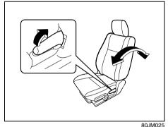
To adjust the seatback angle of front seats, pull up the lever on the outboard side of the seat, move the seatback to the desired position, and release the lever to lock the seatback in place. After adjustment, try moving the seatback to make sure it is securely locked.
