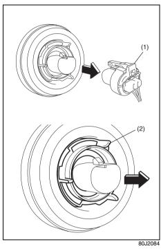
Open the engine food. Disconnect the coupler (1). Then remove the socket cover (2) and replace the bulb. Install a new bulb in the reverse order of removal. (1) Removal(2) Installation
