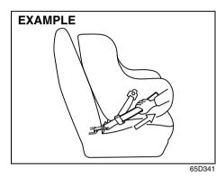
Return the seatback to the normal, upright position. Tighten the lower straps as described in the child restraint owner's manual. Attach the top tether strap, if applicable.
