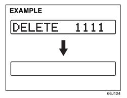
Input your PIN. The power of the audio system will turn off and your PIN will be deleted.
