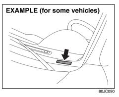
The Vehicle Identification Number (VIN) may be found in the location shown in the above illustrations. This number is used to register the vehicle. It is also used to assist your dealer when ordering parts or referring to special service information.
