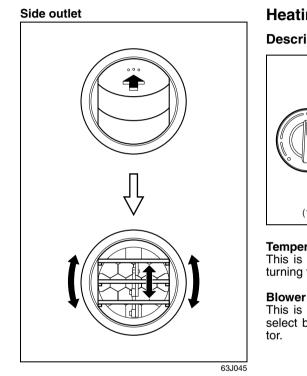
When "Open", air comes out regardless of the air flow selector position.
