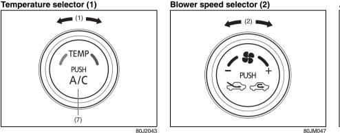
Turn the temperature selector (1) to adjust the temperature.
