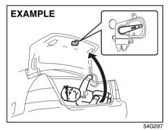
There is a release lever located inside the trunk, on the rear part of the trunk lid. This lever is for emergency use so that if a person, such as a child, gets trapped in the trunk compartment, he can exit the vehicle. The lever glows in the dark, after a brief exposure to ambient light, so it can be found easily. It is operated by pushing it down in the direction of the arrow.
