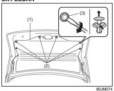
To open the trim (1), insert a flat blade screwdriver into the hole (3) and remove the clips (2) by twist the driver as shown in the illustration.
