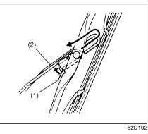
Squeeze lock lever (1) towards wiper arm (2) and remove the wiper frame from the arm as shown.
