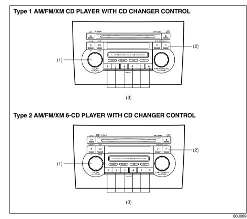
(1) Power on/off knob(2) Track up button/Fast forward button(3) Preset buttons (1 to 6)
