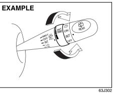
If the lever is equipped with the "INT TIME" control, turn the control forward or rearward to adjust the intermittent wiper operation to the desired interval. Windshield Washer
