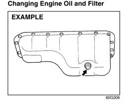
Drain the engine oil while the engine is still warm.
