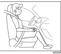
When seated as shown in the above illustration, the front passenger sensing system senses a properly-seated occupant and enables the air bag.
