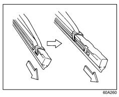
3) Pull the locked end of the wiper blade firmly to unlock the blade and slide the blade out as shown.
