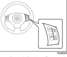
The cruise control system allows you to maintain a steady speed without keeping your foot on the accelerator pedal. The controls for operating the cruise control system are on the steering wheel.
