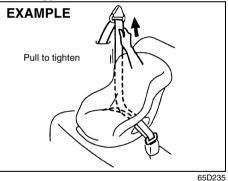
Try moving the child restraint system in all directions, to make sure it is securely installed. If you need to tighten the belt, pull more webbing toward the retractor. Supplemental Restraint System (advanced air bags): 3, 9, 12
