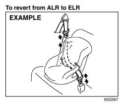
When you unbuckle the seat belt and allow it to retract to a certain length, the retractor will automatically revert back to the normal ELR mode.
