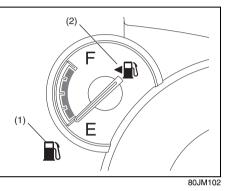
When the ignition switch is in the "ON" position, this gauge gives an approximate indication of the amount of fuel in the fuel tank. "F" stands for full and "E" stands for empty.
