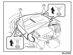
Remove the air cleaner inlet hose (1). Remove the front part (2), then remove the rear part (3) of the air cleaner case.
