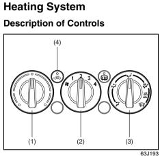
Temperature selector (1) This is used to select the temperature by turning the selector.
