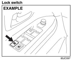
The driver's door also has a lock switch for the passenger's window(s). When you push in the lock switch, the passenger's window(s) cannot be raised or lowered by operating any of the switches (2), (3), (4) or (5). To restore normal operation, release the lock switch by pushing the switch again.
