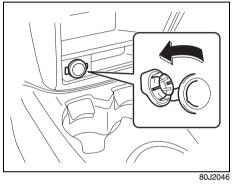
The accessory socket will work when the ignition switch is in the "ACC" or "ON" position.
