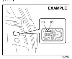
When you open the tailgate with the luggage compartment light switch in the "ON" position (1), the light comes on and remains on as long as you keep the tailgate open.
