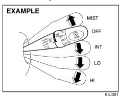
To turn the windshield wipers on, move the lever down to one of the three operating positions. In the "INT" position (if equipped), the wipers operate intermittently. The "INT" position is very convenient for driving in mist or light rain. In the "LO" position, the wipers operate at a steady low speed. In the "HI" position, the wipers operate at a steady low speed. In the "HI" position, the wipers operate at a steady high speed. To turn off the wipers, move the lever back to the "OFF" position.
