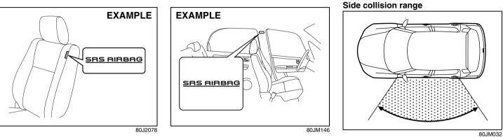
Side air bags are located in the part of the front seatbacks closest to the doors. The words "SRS AIRBAG" are indicated on the tag to identify the location of the side air bags.
