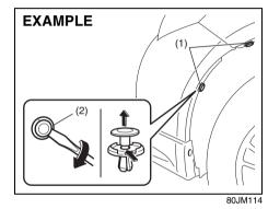
Insert a flat blade screwdriver into the hole (2) and remove the clips (1) by twist the driver as shown in the illustration.
