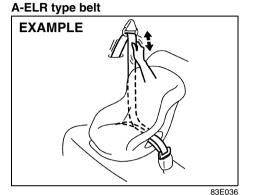
Make sure that the retractor has converted to the ALR mode by trying to pull webbing out of the retractor. If the retractor is in the ALR mode, the belt will be locked.
