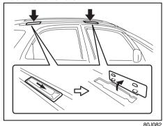
You can use the roof rails or the roof rack anchors to attach the optional roof rack which is available at your SUZUKI dealer. If you use a roof rack, observe the instructions and precautions in this section and provided with the roof rack.
