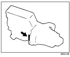
The engine serial number is stamped on the cylinder block as shown in the above illustration.
