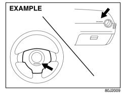
The driver's front air bag is located behind the center pad of the steering wheel and the front passenger's front air bag is located behind the passenger's side of the dashboard. The words "SRS AIRBAG" are molded into the air bag covers to identify the location of the air bags.
