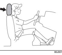
Head restraints are designed to help reduce the risk of neck injuries in case of an accident.
