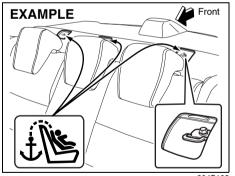
Some child restraint systems require the use of a top strap. Top strap anchor brackets are provided in your vehicle at the locations shown in the illustrations. Install the child restraint system as follows:
