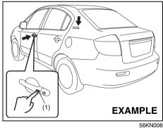
When the remote controller is within the operating range described in this section, you can lock or unlock the doors by pushing the request switch (1) on the door handle of the driver's door, front passenger's door or tailgate of SX4.
