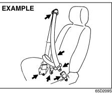
Periodically inspect the seat belts to make sure they work properly and are not damaged. Check the webbing, buckles, latch plates, retractors, anchorages and guide loops. Replace any seat belts which do not work properly or are damaged.
