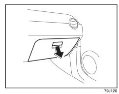
To open the glove box, pull the latch lever. To close it, push the lid until it latches securely.
