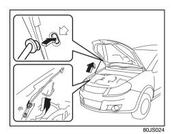
Continue to lift up the hood until it is high enough to support with the prop rod.
