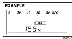
Change the display (B) to the driving range by pushing the indicator selector knob (2).
