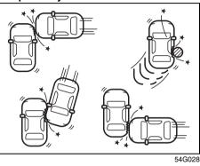
Side air bags and side curtain air bags are not designed to inflate in frontal or rear collisions, rollovers or minor side collisions, since they would offer no protection in those types of accidents. Only the side air bag and side curtain air bag on the side of the vehicle that is struck will inflate. Remember, since an air bag deploys only one time during an accident, seat belts are needed to restrain occupants from further movements during the accident.
