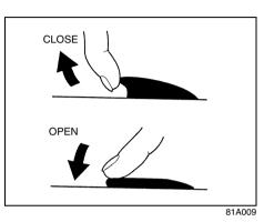
To open a window, push the top part of the switch and to close a window lift up the top part of the switch.
