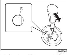
Vehicles with a CVT have an electrically operated park-lock feature. If the vehicle's battery is discharged, or there is some other electrical failure, the CVT cannot be shifted out of Park in the normal way. Jump starting may correct the condition. If not, follow the procedure described below. This procedure will permit changing the transaxle out of Park.
