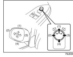
The switch to control the power rearview mirrors is located on the driver's door panel. You can adjust the mirrors when the ignition switch is in the "ACC" or "ON" position. To adjust the mirrors:
