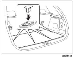
Place the strikers of the luggage board to the latches on the side and tail end of original position.
