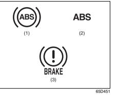
(1) ABS warning light Type 1(2) ABS warning light Type 2(3) Brake system warning light
