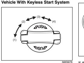
The ignition switch can be operated without using an ignition key when the remote controller is in an area of the vehicle other than the rear luggage area. To turn the ignition switch, first push in the switch.
