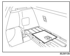
The lid can be installed on the back of the luggage compartment board.
