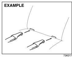
Place the child restraint in the rear seat, feeding the strap hooks through the slots in the seat cushion or the slots in the seatback bottom.
