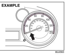
The speedometer indicates vehicle speed in km/h and mph.
