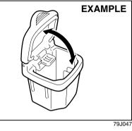
You can fit the ashtray into any of the cup holders on the center console.
