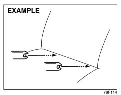
2) Place the child restraint in the rear seat, inserting the connecting bars through the slots in the seat cushion or the slots in the seatback bottom.
