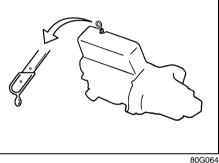
It is important to keep the engine oil at the correct level for proper lubrication of your vehicle's engine. Check the oil level with the vehicle on a level surface. The oil level indication may be inaccurate if the vehicle is on a slope. The oil level should be checked either before starting the engine or at least 5 minutes after stopping the engine.
