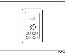
The front fog light comes on when the fog light switch is pushed in with the headlights are on and the beams set to the low beam position.
