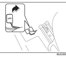
If your vehicle is equipped with a trunk lid unlatch switch (1), push and hold the trunk lid unlatch switch (1) and lift the trunk lid to open the trunk lid.
