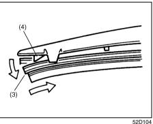
1) Flex the locked end of blade (3) away from retainer (4) to unlock it and slide the blade out as shown.
