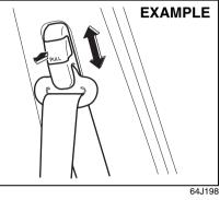
Adjust the shoulder anchor height so that the shoulder belt rides on the center of the outside shoulder. To upward, slide the anchor up. To downward, slide the anchor down while pulling the lock knob out. After adjustment, make sure that the anchor is securely locked.
