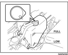
If the engine coolant level is below the "LOW" mark, more engine coolant should be added. Remove the reserve tank cap and add engine coolant until the reserve tank level reaches the "FULL" mark. Never fill the reserve tank above the "FULL" mark.
