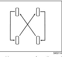
To avoid uneven wear of your tires and to prolong their life, rotate the tires as illustrated. Tires should be rotated as recommended in the periodic maintenance schedule. After rotation, adjust front and rear tire pressures to the specification listed on your vehicle's Tire and Loading Information Label.
