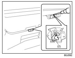
2) Push open the tailgate from inside by pushing up on the emergency lever (2) using a flat blade screwdriver or the jack handle. The tailgate will be latched again by closing the tailgate simply.
