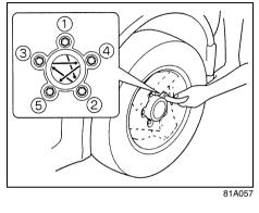
Wheel tightening torque 85 Nm (61.5 lb-ft, 8.5 kg-m)
