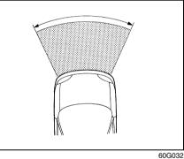
Front air bags are designed to inflate only in severe frontal collisions.
