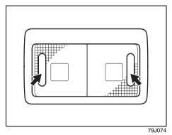
Push the switch to turn on the light and push it again to turn off the light.
