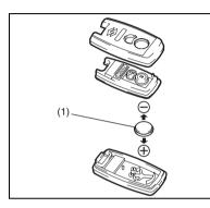
(1) Lithium disc type battery: CR2032 or equivalent
