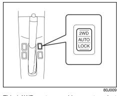
This i-AWD system enables you to select the driving mode according to the driving conditions by operating the 2WD/i-AWD switch. With this feature, you can select 3 mode positions, "2WD", "i-AWD AUTO" and "i-AWD LOCK" by operating the 2WD/ i-AWD switch even when the vehicle is moving, provided the front wheels are in the straight ahead position.
