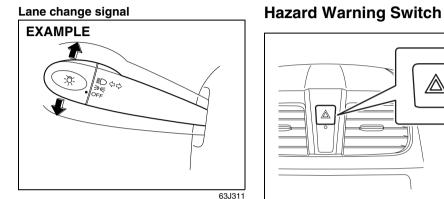
Some times, such as when changing lanes, the steering wheel is not turned far enough to cancel the turn signal. For convenience, you can flash the turn signal by moving the lever part way and holding it there. The lever will return to its normal position when you release it.
