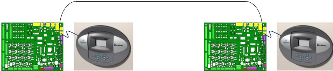
**Three or more units with small displays:** To network three or more cooling units, each equipped with a small display, connect a straight-through CAT5 Ethernet cable from the P64 connector on each cooling unit's Liebert iCOM input/output board to a common network switch (see **Figure 26**).
