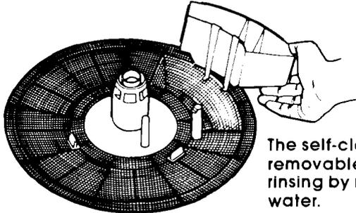
The self-cleaning filtering system and removable pump guard help eliminate pre-rinsing by removing food particles from the water.
