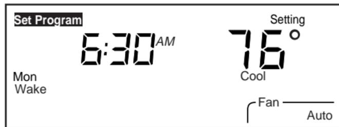
By pressing **Increase ▲** or **Decrease ▼**, you select the cooling Wake temperature. Example display shows the cooling Wake period set for 76°.
