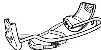
Lower Swing Arm Assembly (with Restraint System)
