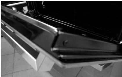
Remove screws from both side of door
