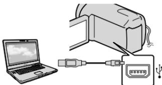
The [USB SELECT] screen appears on the camcorder screen automatically.
