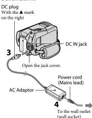
You can charge the "InfoLITHIUM" battery pack (H series) (p. 91) after attaching it to your camcorder.
