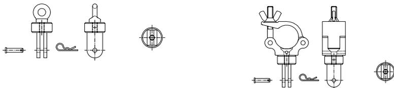
The **SC-440 aluminium scaffold clamp** is attached to the T-bar by means of a simple clevis coupler. It is designed to rotate horizontally through 360° in order to enable accurate positioning of the loudspeaker. The point at which the scaffold clamp is attached to the flybar determines the vertical angle of the loudspeaker as shown in the table following.
