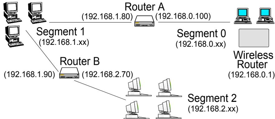
Figure 45: Routing Example
