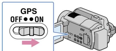
Set the GPS switch to ON (
