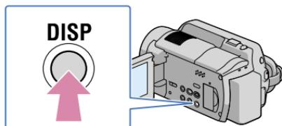
Each time you press DISP, the screen indicators, such as remaining battery power, etc., turn on or off.
