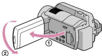
Open the LCD panel 90 degrees to the camcorder ①, then rotate it 180 degrees to the lens side ②.
