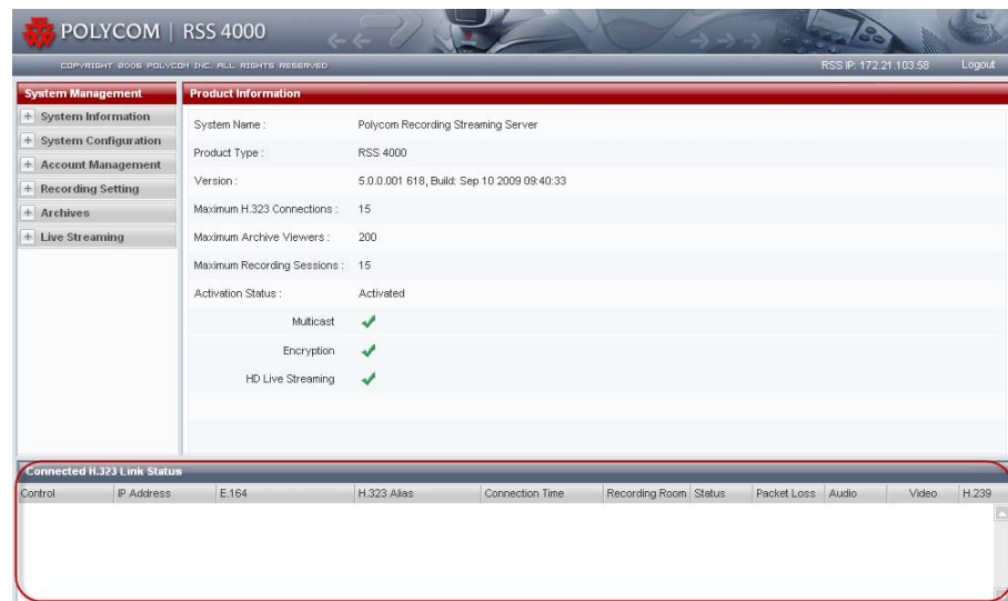
Figure 2-45 H.323 Connection Status Display Area
