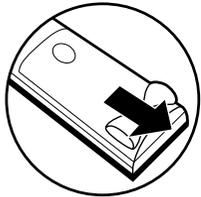
② Insert two "AA" (R6) batteries, with each one oriented correctly.
