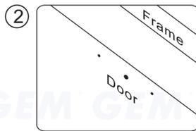
2 Drill three holes in the door as indicated on the template.
