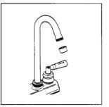
4 Unscrew aerator from the end of the spout. Turn on hot and cold water to flush lines and faucet. Turn faucet off and replace aerator.
