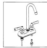
Connect hot and cold supply lines onto faucet shanks with coupling nuts. FINGER tighten securely.
