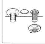
From underside of sink fasten faucet with plastic mounting nuts. FINGER tighten securely. DO NOT OVER TIGHTEN.
