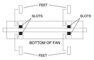
WARNING: MAKE SURE FEET ARE NOT ATTACHED WHEN USING FAN IN A WINDOW.
